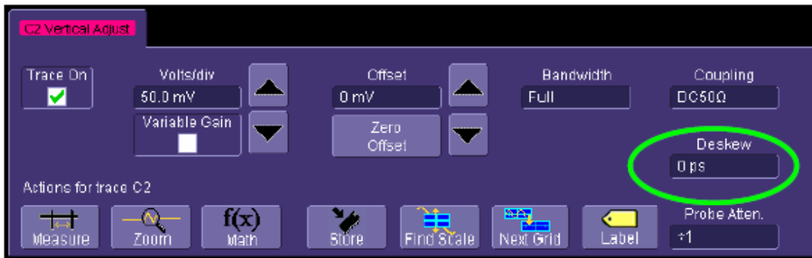
Deskew control in channel menu. Adjust this value to achieve minimum skew.
